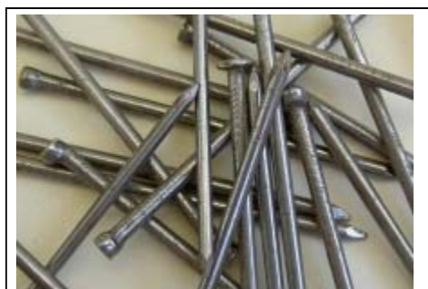
Iron nails are nonmagnetized materials. However, they have the potential to be magnetized.
