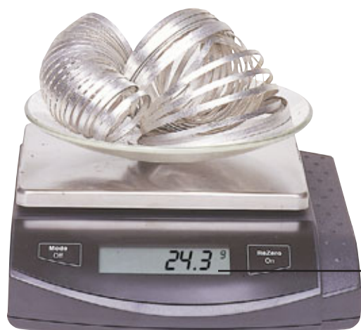
Figure 7 One mole of magnesium ( 6.022 \times 10^{23} Mg atoms) has a mass of 24.3050 g. Note that the balance is accurate only to one-tenth of a gram, so it reads 24.3 g.
